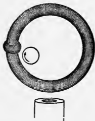
FIG. 127.—Magnetic Leakage across a Throttled Iron Ring, causing rotation of an Iron Disc placed near the Secondary Coil.
